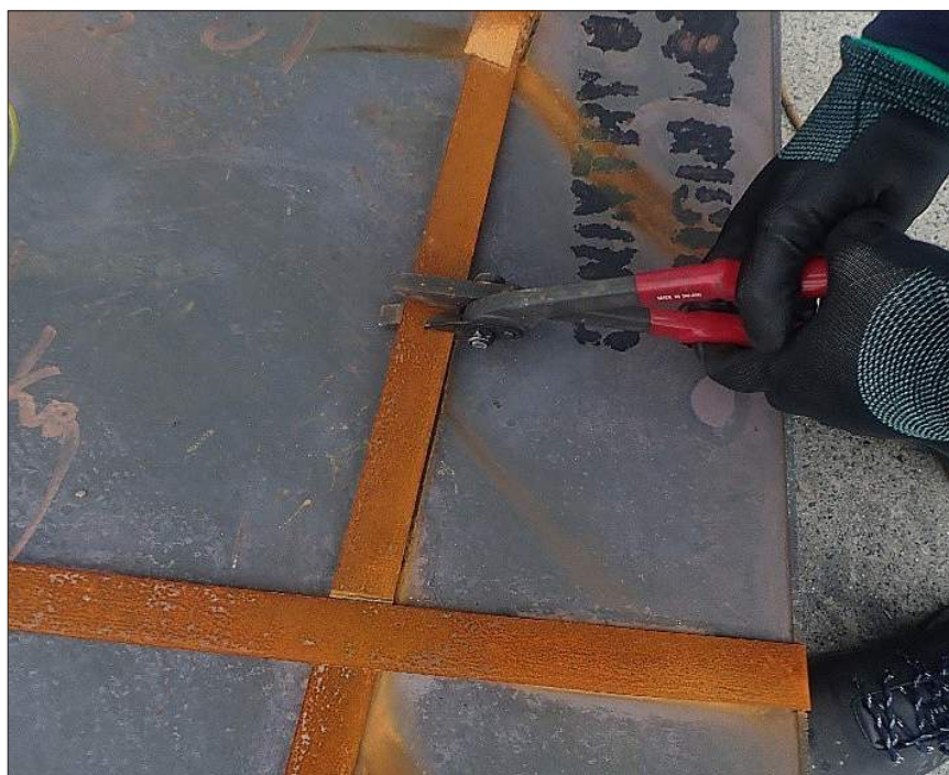
Figure 1. Copper cathode plates contaminated by steel band straps. © The authors
