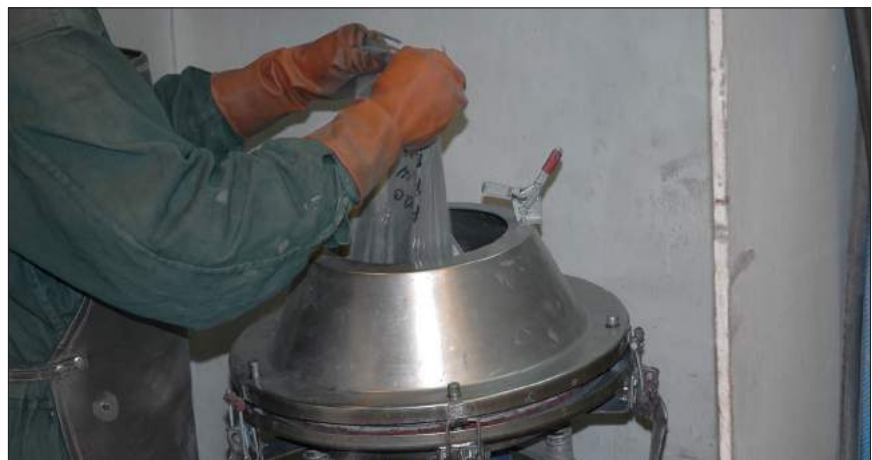
Figure 1. Screen fire assay is always a good option in the presence, or suspected presence, of coarse gold. It provides a good spatial measure of the problem. It is important to ensure that a nylon screen is used that is fire assayed to extinction. This removes sample-to-sample contamination of the screen. Duplicate or triplicate fire assays should be applied on the undersize fraction to check the level of heterogeneity—some “fine” coarse gold can still pervade the fine fraction.
