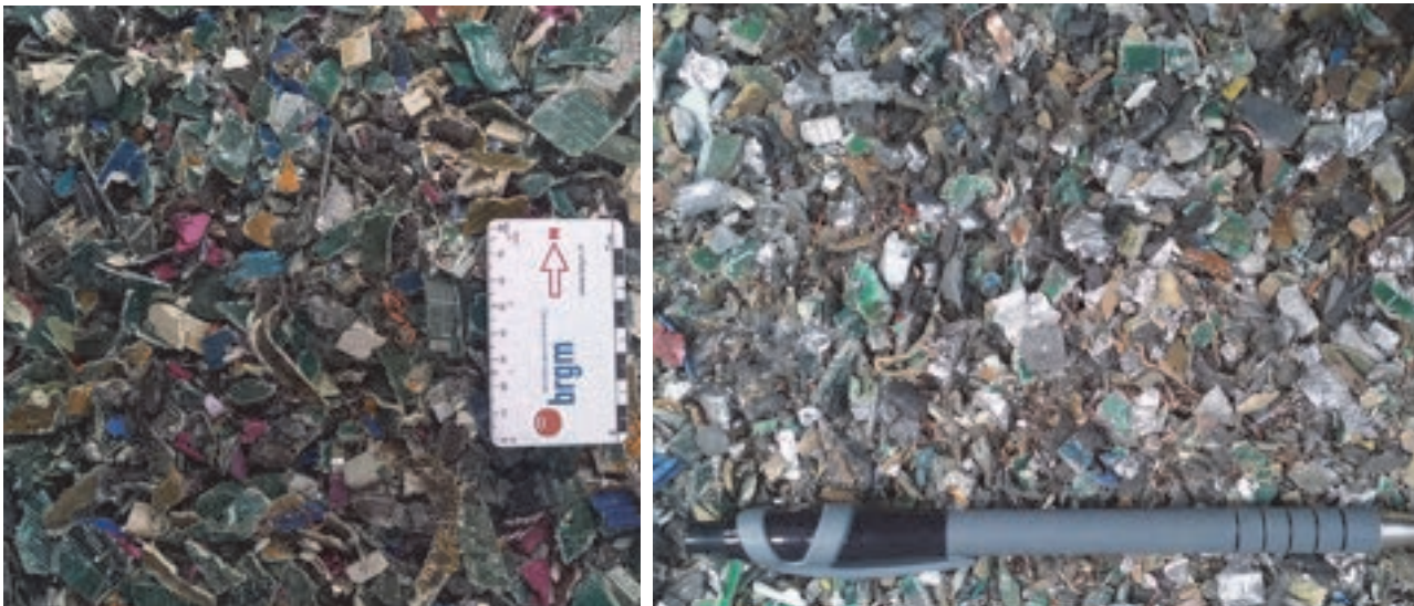
Figure 2. The lot of WPCB after shredding to -30 mm (left) and a quarter of that lot after shredding to -10 mm (right).
