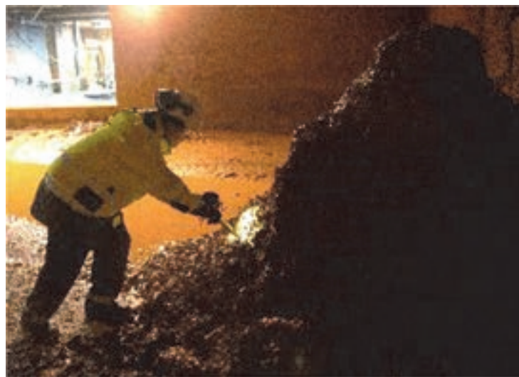
Figure 6. Illustration of spear sampling the iron sludge pile at ground level.
