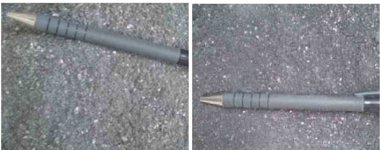
Figure 3. 4 kg sample of WPCB shredded to -2 mm (left) and another 4 kg sample shredded to -750 µm (right).
