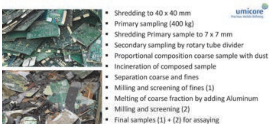
Figure 8. Sampling of e-scrap @UPMR
