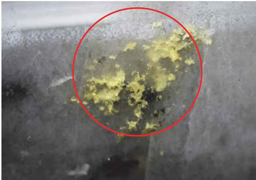
Figure 3. Coarse gold cluster in sulphide-poor (Early phase) mineralisation from VC drill core. Width of cluster on core surface c. 20 mm (red circle).
