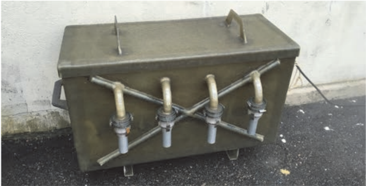
Figure 2. The sampling device is about 1 m long by 0.40 m tall. The unit can be moved easily with a forklift or manually.
