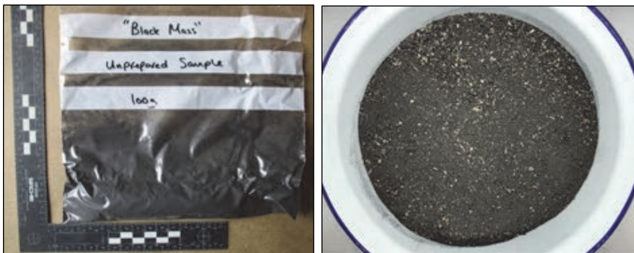
Figure 4. Unprepared sample of black mass submitted for analysis (left). The diameter of the sample dish (right) is approximately 150 mm.
