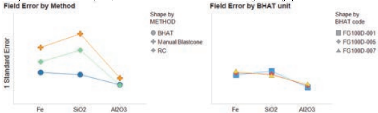
Figure 1. Summary results for different methods of assay data acquisition at a mining site (left). Note the high error for manual blastcone sampling using shovels and the lowest error for the BHAT method. The plot on the right shows field error for three BHAT units operating at the mine site, showing consistent results. Note: One Standard Error is given as the standard deviation of the absolute difference between sample pairs.
