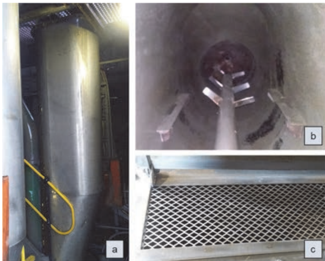
Figure 2. Day Tank – a. Oval Tank Design; b. Off Centre Agitator inside Day Tank; c. Sampler Inspection/Safety Grid.
