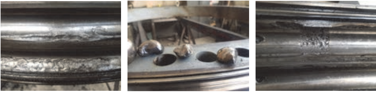
Figure 9. Appearance of blade bearing B, a deep groove ball bearing. Note the heavy peeling on the raceway and that several of the balls were cracked.
