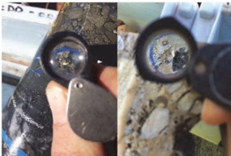
Figure 2. Gold in drill core from fresh conglomerate, Grants Hill. Left: BCDD18-002, 0.5 m at 7.3 g/t Au. Right, BCDD18-001, 0.48 m at 4.3 g/t Au.
