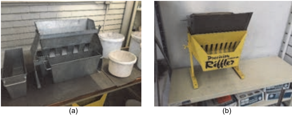
Figure 4: (a) Riffle splitter for coarse materials, >10 mm, and (b) riffle splitter for fine materials, <10 mm Following the splitting process, the samples are bagged (Figure 5a), weighed (Figure 5b), and prepared for dispatch to the analytical laboratories (Figure 5c).
