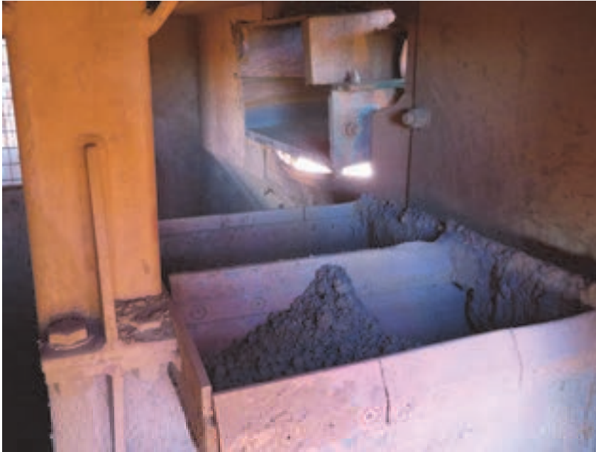
Figure 11. Sample build-up in the secondary cutter apertures.
