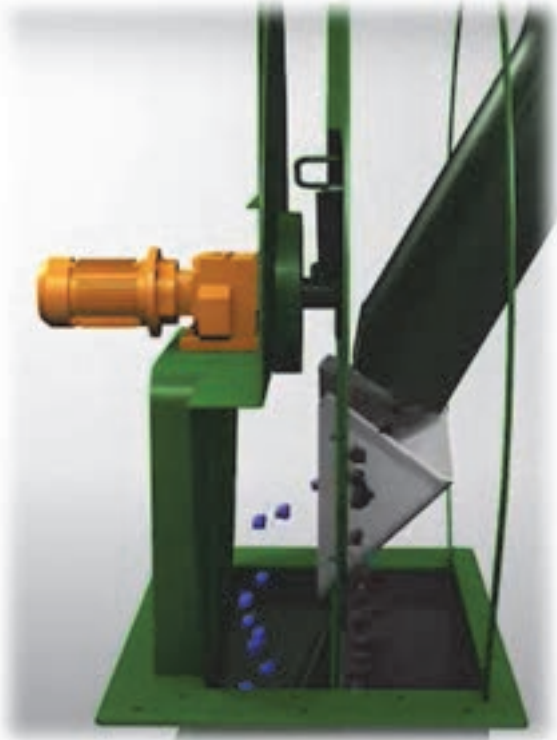
Figure 3. Sectional view of the Rotating Plate Divider feed pipe (on the right) presenting a sample increment to the cutter (middle) to sub-sample (blue particles) the stream and generate rejects (black particles) on the feed side of the plate. Sample and rejects report to separate, isolated chutes.
