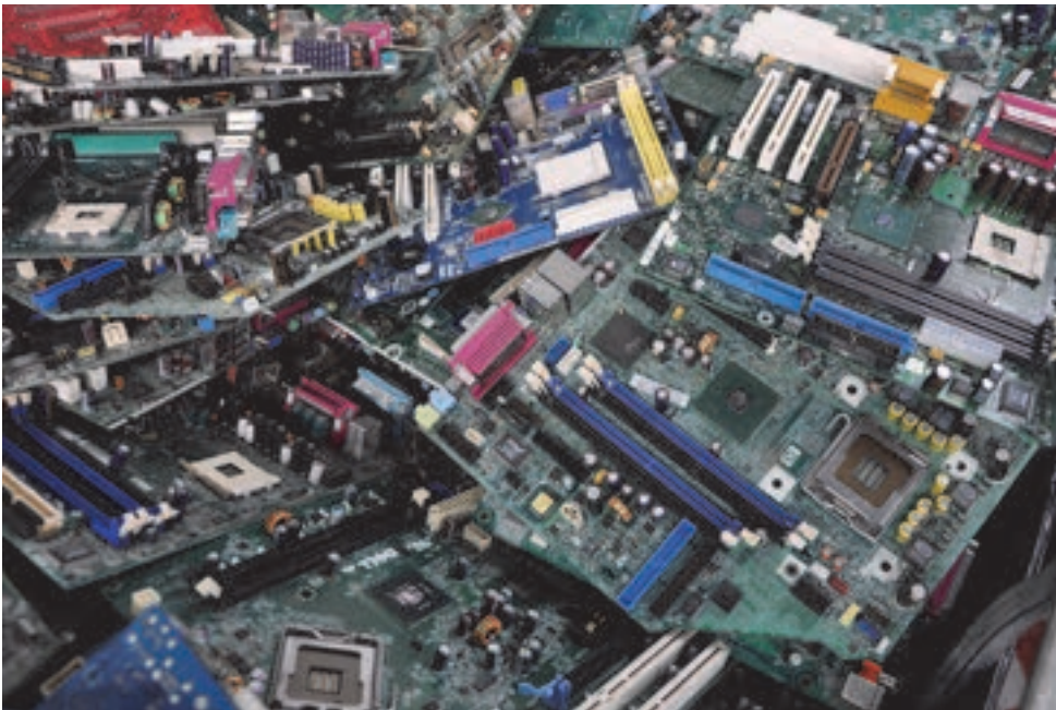
Figure 1. A lot of WPCB illustrating the high heterogeneity of the material to be sampled.
