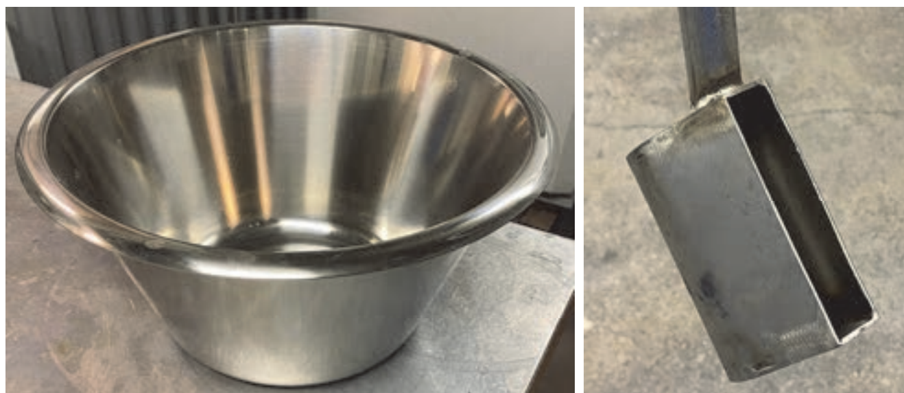
Figure 2. Left: Container used to collect material from the Scavenger Tailings and Final Concentrate sampling locations. Right: Manual sample cutter used for sampling Rougher Tailings, with a cutting aperture of 18 mm.
