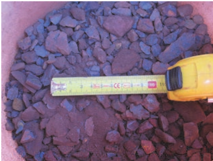
Figure 8. Nominal top size check of crusher product in a sample station. In this case the target nominal top size of 10 mm was not achieved.
