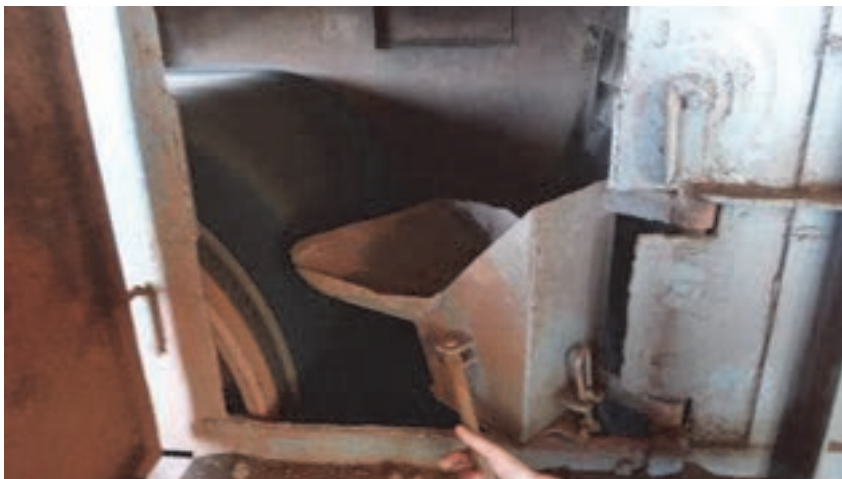
Figure 3. Poorly designed primary cutter that pivots around an axis on the side of the conveyor belt, so the cutting time at each point in the stream is not equal.
