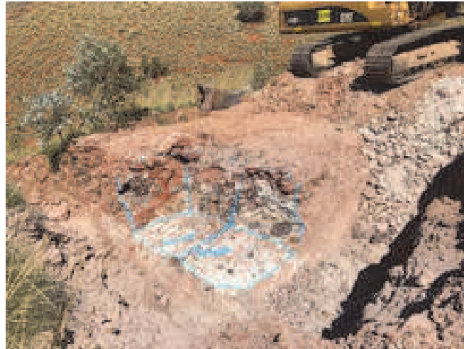
Figure 5. Tightly packed armored lag-type oxide conglomerate with quartz boulders from the M1 reef, Edwards area.
