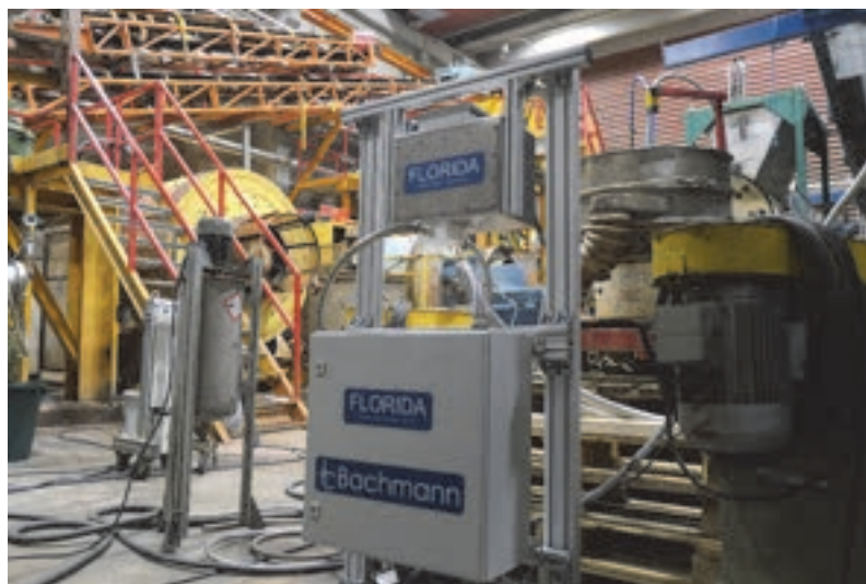
Figure 1. FLORIDA XRF analyser that has been installed at a flotation cell of the GTK Mintec plant for our experiments. The upper box of the device is the sensor head consisting of an X-ray tube, an SDD detector, and a cooling system. It is fed by the attached pipe. The lower box contains the control cabinet of the device.
