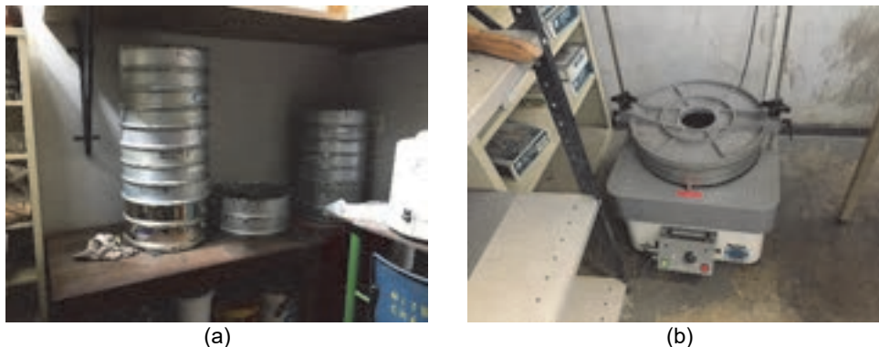
Figure 1: (a) Nested screens for separating ores into correct size fractions, and (b) the mechanical sieve shaker. The distribution of the mass for each of the screened size fractions is shown in Figures 2a and 2b for the Wessels and Mamatwan mines, respectively.
