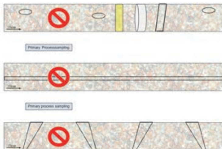
Fig. 2. Key commonality between physical increment/sample volume and sensor signal support in process sampling: Identical rules apply w.r.t. correct increment delineation and extraction (complete and undisturbed volumetric coverage) for both physical extraction as well as for delineation of the sensor signal support volume as facilitated by a sampling interface. This illustration can either be viewed as looking down on a heterogeneous 1-D moving material lot f.ex. on a conveyor belt - or it can be understood as a vertical section through a horizontal conduit transporting a heterogeneous material (indicated by irregular texture). From both points of view, TOS-correct process sampling necessitates recovery of, or spectral coverage of, the full delineated cross-stream increment volume, shown by the three renditions in the upper panel Only fully covering increment volumes with planar-parallel boundaries will result in representative increments or samples. Illustration copyright KHE Consulting teaching collection, used with permission.
