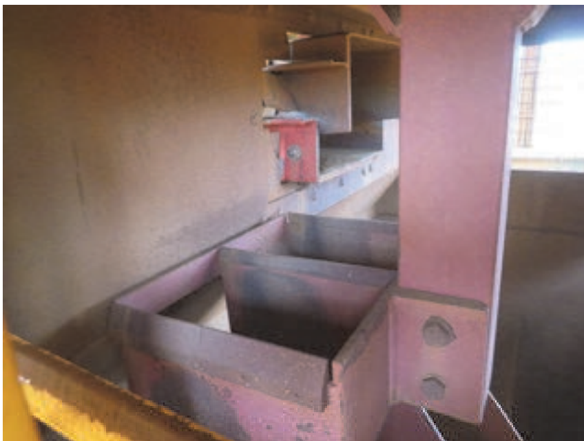
Figure 7. Cross-stream secondary cutter designed to collect separate increments for chemical/moisture analysis and sizing.
