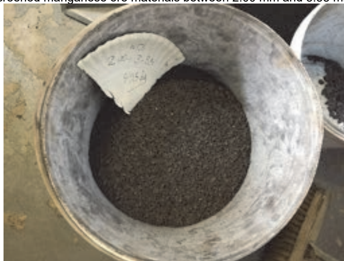
Figure 6: Closely screened manganese ore materials between 2.00 mm and 3.35 mm, with an average d_N = 2.659 mm The average nominal top-size of a fraction retained between screens of 1.266 cm and 0.63 cm is calculated as follows:
