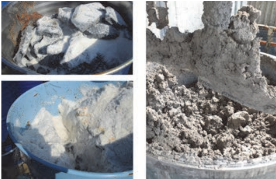
Figure 12. Filter Cake with white sand – Mixing result
