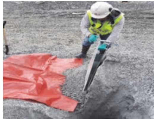
Figure 5. Fabricated sectional metal frame used for the investigation to collect a complete profile through the cone of drilling chips
