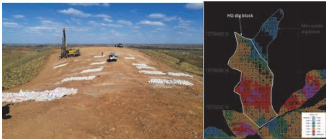
Figure 20. RC grade control drilling and sample bags awaiting laboratory submission (L) and grade control block model dig plan (R).
